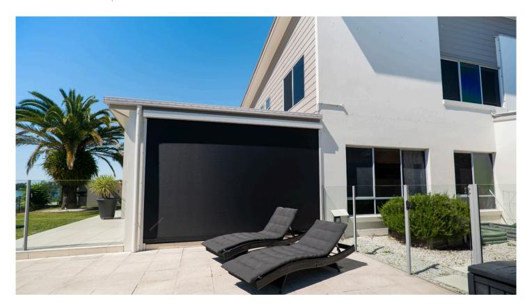
ZIP X is a side-retained product featuring a double spline that smoothly guides the screen into its side channel, ensuring efficient operation. Its streamlined side channels offer an uninterrupted view, maintaining structural integrity to support dimensions up to 5.3 meters in width and 3 meters in drop without needing posts (recommended maximum dimensions). The well-engineered bottom rail prevents bowing and deflection, ensuring durability and performance.
